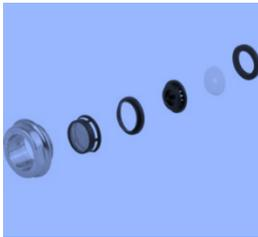
**Disassemble the aerator.** Take out the washer or O-ring and push the internal parts or just the one part out of the aerator housing. \*Remember how it is assembled so you can reassemble after cleaning. A small paper clip or pin might help if there is more than one part to the aerator. If the components are stuck, soak the aerator in white vinegar and warm water (one part vinegar to one part water) or lime-dissolver solution for 30 minutes.
