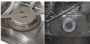
**Clean the dishwasher trap:** Down in no-man's land, under the lower sprayer, there is usually a part or screen that is removable. Under it you will usually find bits of food that did not make it out the drain. Sometimes the tray or screen comes out completely so it can be rinsed in the sink. Sometimes a towel is needed to remove any gunk buildup.
